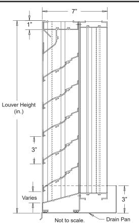
Louver Width O.D. of Drain Pan
